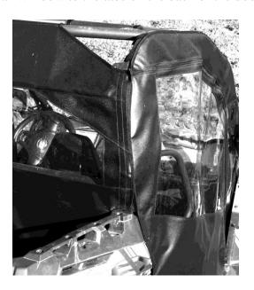
6. The bottom of the Rear Window is held in place by 4 snaps. Photo below shows how this should go.
