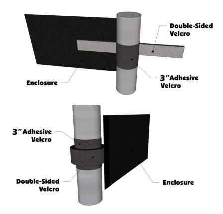
2. Next take the 20" adhesive Velcro strips and run it down the back of the roll cage facing towards the rear of the vehicle. Start at the bottom and work your way up the bar. You will see the double-sided Velcro tabs sewn along the back of the doors. See photo below.
