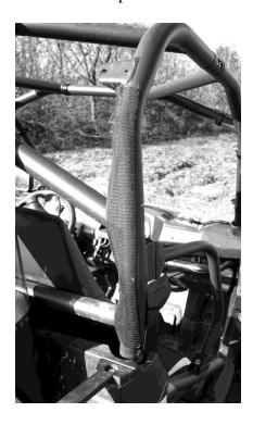
3. Once all the Velcro is in place the last thing to do is install the screw snap studs. NOTE: **The best way** to install the snap studs is to put them in the sockets in the door first. Then push them into the
