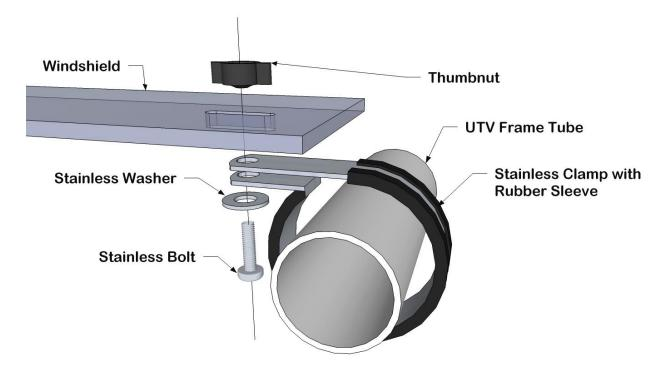
7. The four clamps that hold the windshield across the top use the large stainless and rubber washers to hold the windshield on. The inside part of it uses a small washer and a lock nut. the following photo shows how it should look.
